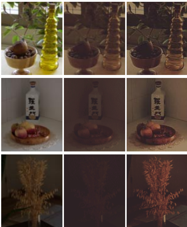
Figure 4. Result images. The first column shows the original images. The second one contains the original images viewed on a simulated transfective display. The third column consists of enhanced images viewed on the same display.
