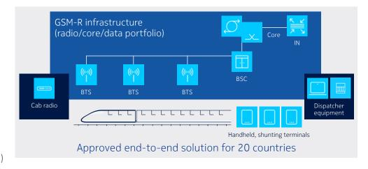
and integrating GSM-R solution components. Now all GSM-R interfaces are standardized, operators have access to an open, interoperable and international system that brings considerable savings.
