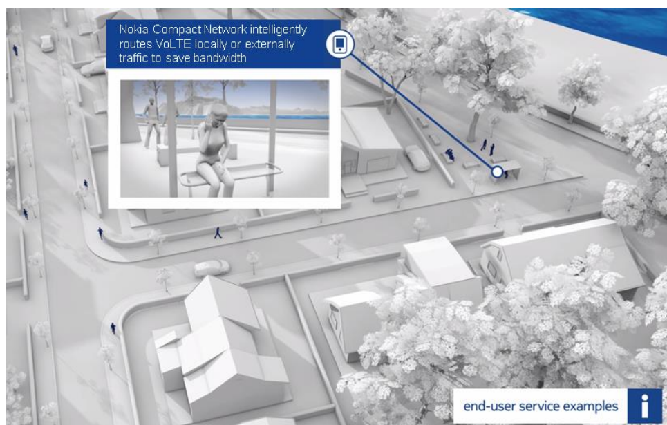
Figure 4. Locally routed voice traffic with Nokia Compact Network in remote hot spots areas
