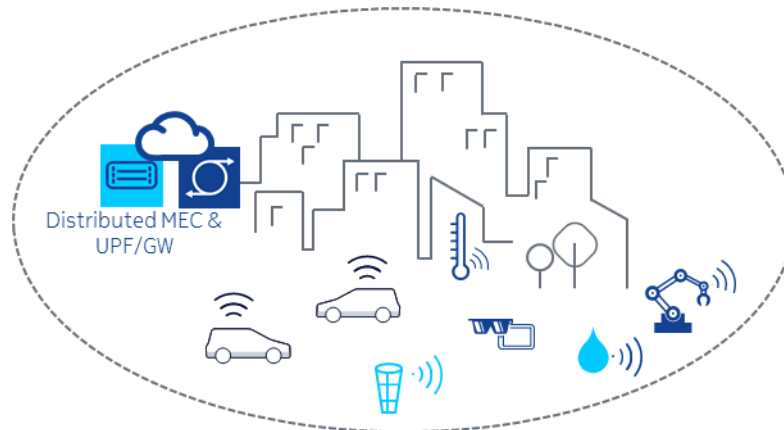
Figure 3. Distributed MEC city edge deployment to provide high availability, support many simultaneous users (potentially millions), transfer large amounts of data and support ultra-low latency services
