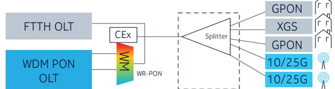
Scenarios 2 is currently the most prominent solution. While scenario 4 has some deployment already for LTE, scenario 3 is being heavily investigated for future deployments. The use of TDM PON and P2P WDM PON are shown for both the case of a dedicated fiber in a common cable and a dedicated wavelength in a common fiber. (in Figure 2, CEx is a coexistence element and WM is a wavelength multiplexer)
