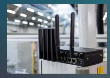
Fieldrouters ruggedized for industrial environments, vehicles and outdoor use, support a wide range of licensed and unlicensed bands in 4G, 5G and MulteFire with a comprehensive feature set to enable efficient traffic for PROFINET communication and other protocols, like EtherCAT and Modbus.
