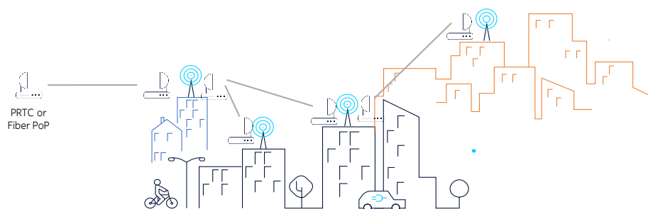
Figure1. E2E synchronization distribution via a microwave transport network
