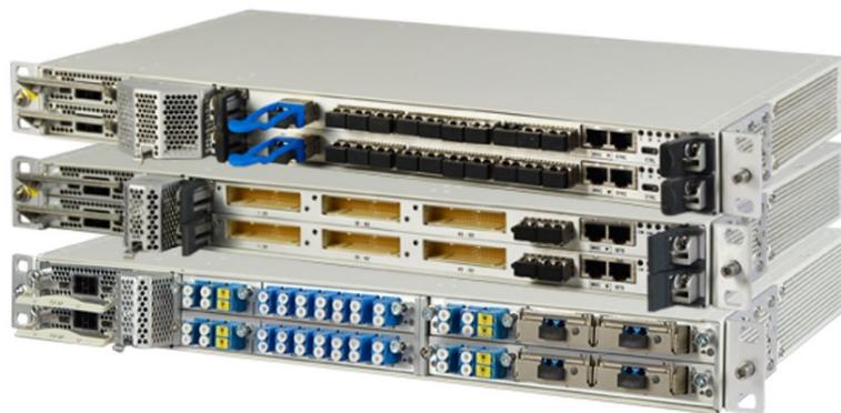
granularity. The 100G OTN switching cards support both B&W (QSFP28) and coherent (CFP2 DCO) interface options. To improve flexibility, the ports on the OTN switching cards can be provisioned as client or line interfaces depending on the configuration needed.
