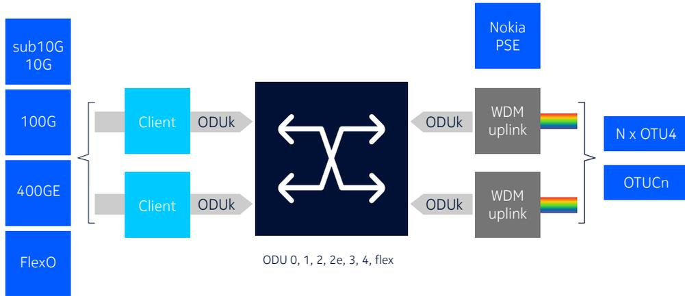
**Figure 6. Distributed OTN switching with 1830 PSS-8 and S13X100**
