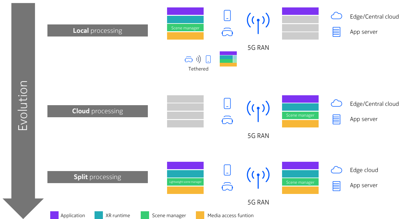
Figure 5. XR processing from device to cloud
