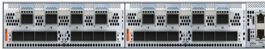
Figure 4: Nokia 1830 GX G31 with two SPN2s and 2.4T (2 x 1.2T) OTN switching configuration
