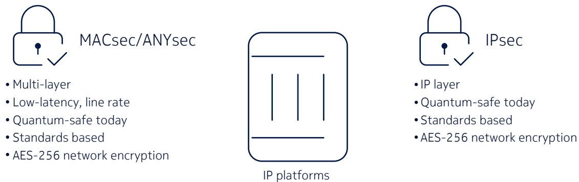
Figure 8. Quantum-safe IP cryptographic technologies
