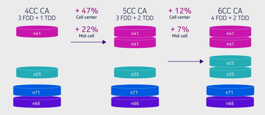
Performance enhancements in the cell center and mid-cell when comparing 4CC CA, 5CC CA and 6CC CA in T-Mobile's commercial production network. On the next page, we describe the 6CC CA field tests in more detail.
