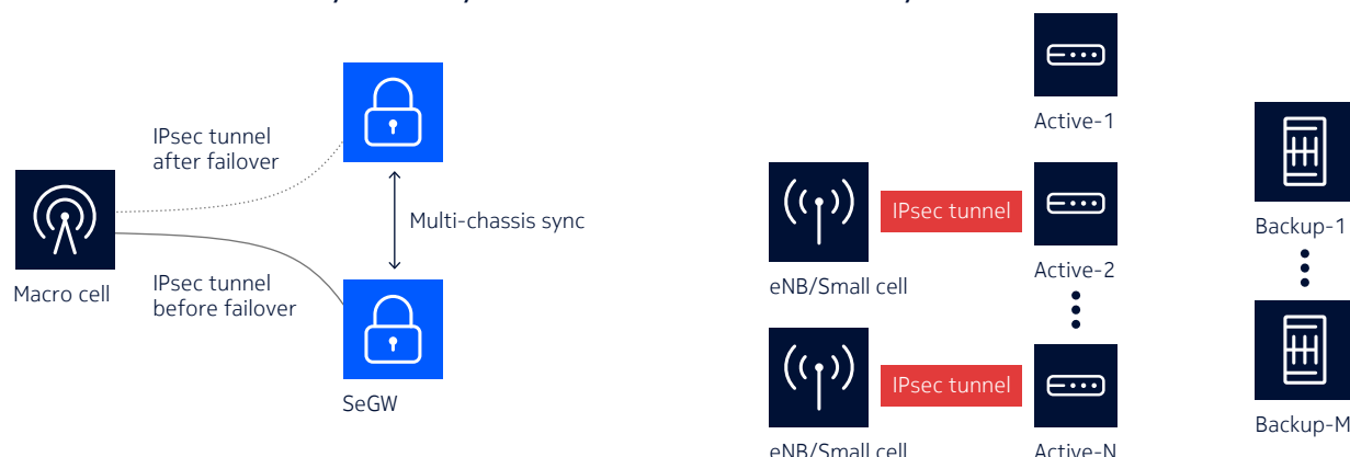
Figure 7. Nokia IPsec Security Gateway N:M multi-chassis redundancy
