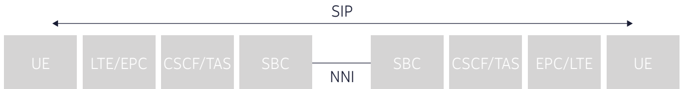
Figure 8. VoLTE interconnect links CSP networks to ensure that calls stay on the IP infrastructure
