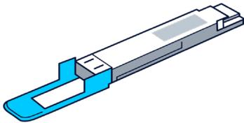
Figure 1. 400ZR module in a QSFP-DD form factor
