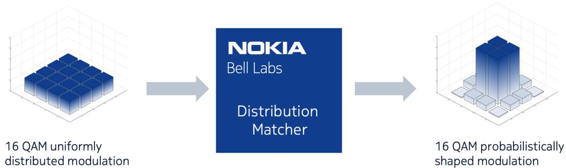
Figure 5 Nokia's patented distribution matching algorithm shapes a uniformly distributed square constellation into a probabilistically shaped constellation
