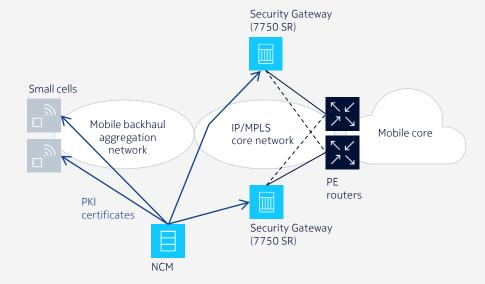
The Nokia Security Gateway provides the industry's highest capacity and throughput. Each security gateway can support 500,000 tunnels for small cells, including femtocells.
