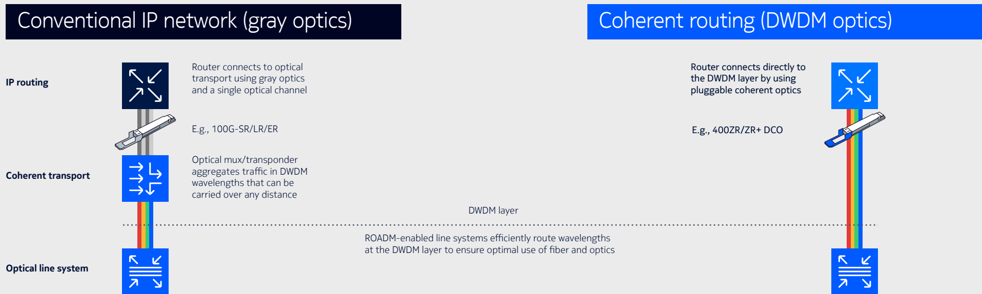
Figure2. Coherent routing: IP-optical transport for 400GE and beyond
