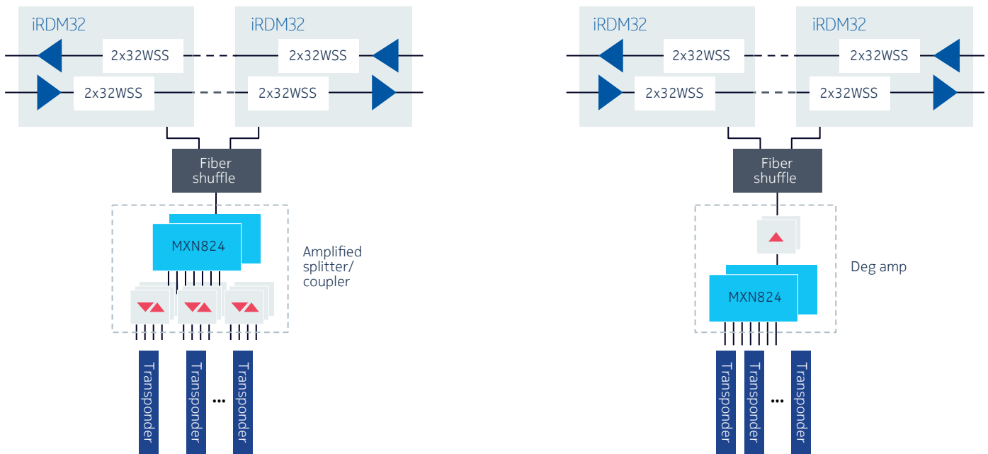
Figure 5a) Amplified splitter/coupler and 5b) WSS Degree Amplifier
