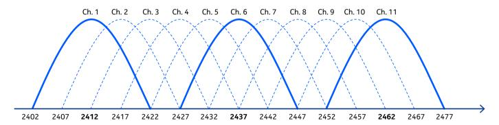
If you want to use 40 MHz channel width in the 2.4 GHz band, then only one non-overlapping channel can be used.
