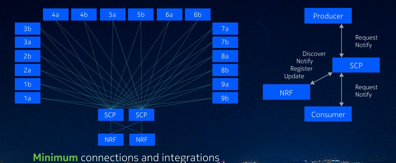
Model D is only proposed by vendors with a fully capable SCP. This is the target architecture for nearly all 5G service providers.
