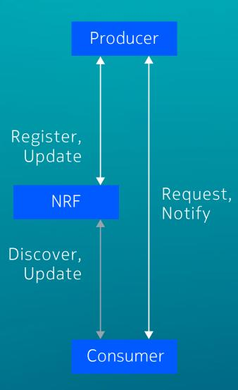
The NRF is the database that maintains the record of available NFs and their supported services. Without it, the core reverts to a peer-to-peer architecture with fixed connections between the NFs.
