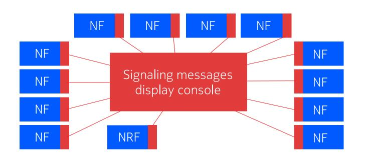
Individual probe for every network function to decrypt messages for each signaling link
