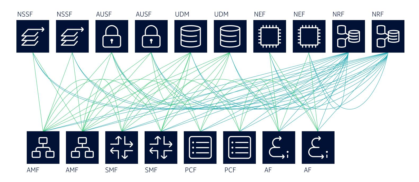
The SBI bus in reality consists of many point to point connections between network functions.
