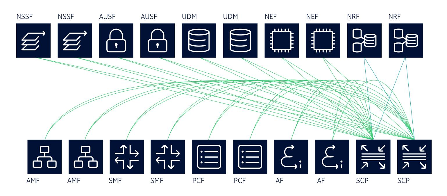
Since the SCP was introduced only in 5G Release 16 (Rel-16), CSPs who deployed 5G Standalone (SA) core prior to this release did not have the option to include an SCP. But nearly all CSPs today plan to move to a full SBA approach with the SCP.
