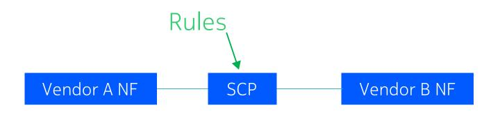
Protocol mismatch adapted by rules engine in the SCP on the fly
