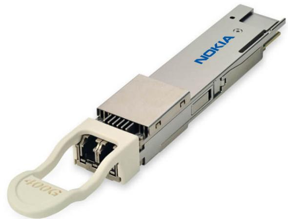
400G/16QAM mode, depending on optical link characteristics, 400ZR+ can achieve distances up to 600 km with external amplification. Even greater distances are possible when operating at sub-rates below 400G using QPSK or 8QAM modulation. Additionally, 400ZR+ can traverse a limited number of reconfigurable optical add-drop multiplexer (ROADM) nodes, enabling efficient router bypass when necessary.
