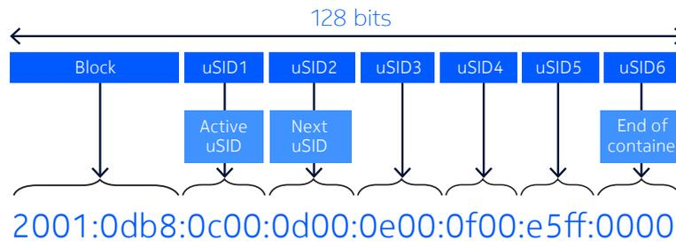
A 32-bit uSID-Block (Locator Block) supports the encoding of up to six 16-bit uSIDs. In the example shown in Figure 3, the container encodes five 16-bit uSIDs plus an end of container marker using a special uSID value of '0000'.
