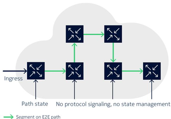
Segment routing leverages the IPv6 data plane using a routing header called the Segment Routing Header (SRH). SRv6 SIDs are encoded as IPv6 addresses. A segment list can be formed from a single segment or an ordered list of segments within the SRH.
