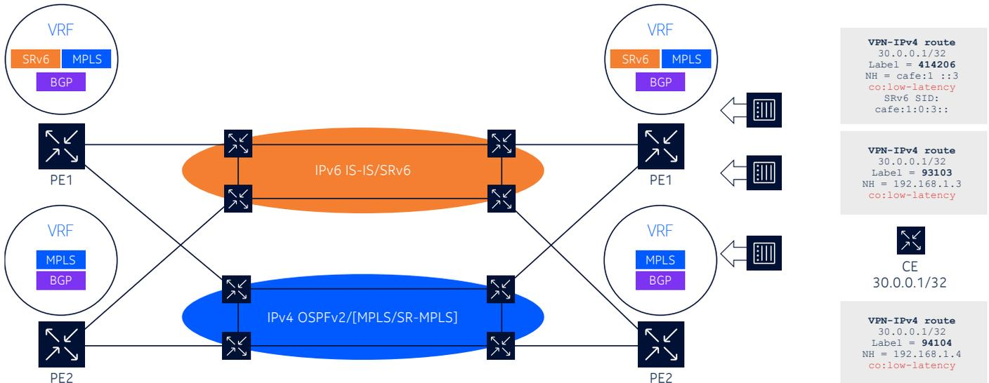
In Figure 7, an MPLS provider edge (PE) router advertises a customer edge (CE) router as a MPLS VPN route with a service label. It can only resolve an imported remote CE MPLS VPN route to an SR-OSPF tunnel.
